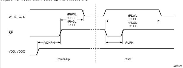
Figure 18. Reset and Power-up AC Waveforms
