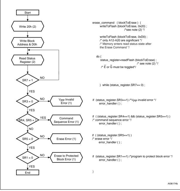
Note: 1. If an error is found, the Status Register must be cleared before further Program/Erase operations. 2. Any address within the bank can be used also.
