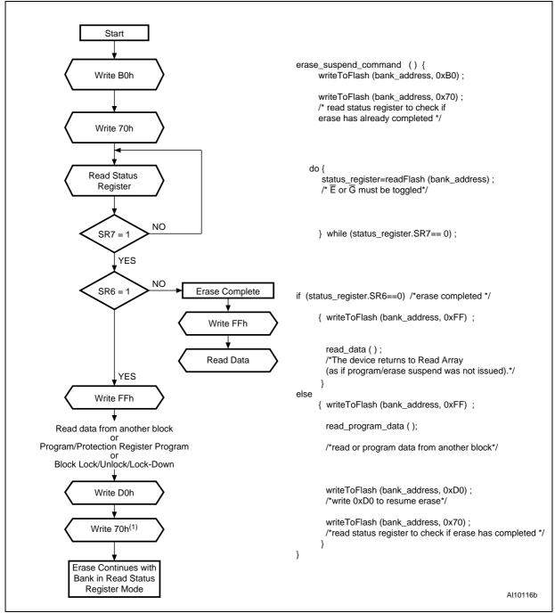
Figure 27. Erase Suspend & Resume Flowchart and Pseudo Code
