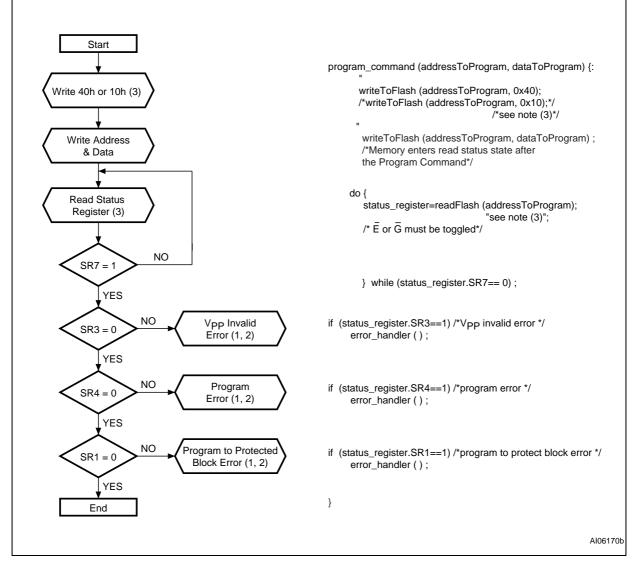
Note: 1. Status check of SR1 (Protected Block), SR3 (VPP Invalid) and SR4 (Program Error) can be made after each program operation or after a sequence.
